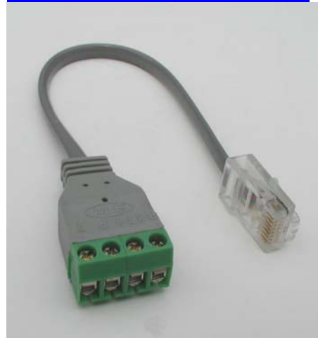
(BM-BW8) Panel phone line input adapter for alarm panels with female RJ-45 inputs instead of screw terminals
